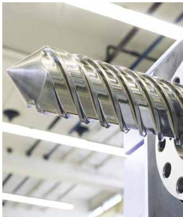
The core of any extruder: the screw.
