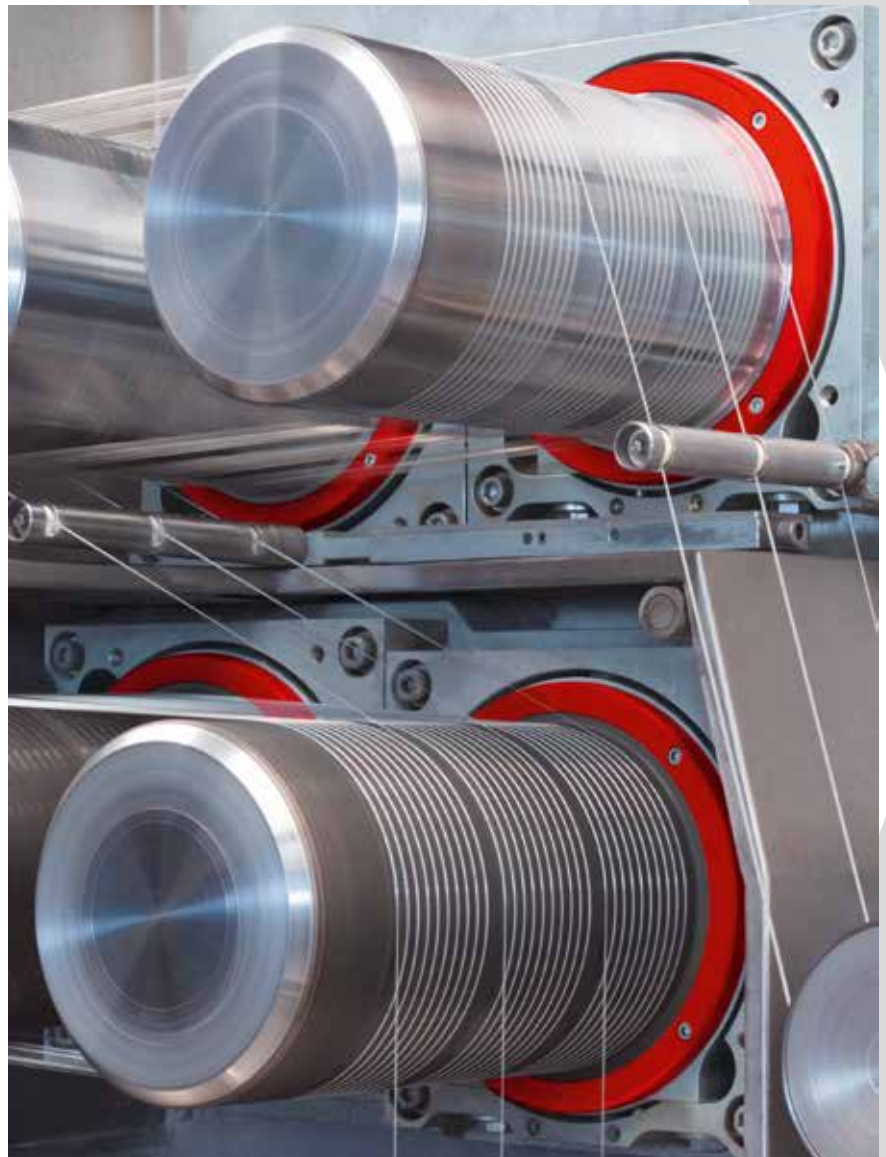
The absolutely straight yarn path from the infeed to the cooling drum improves the production process.
