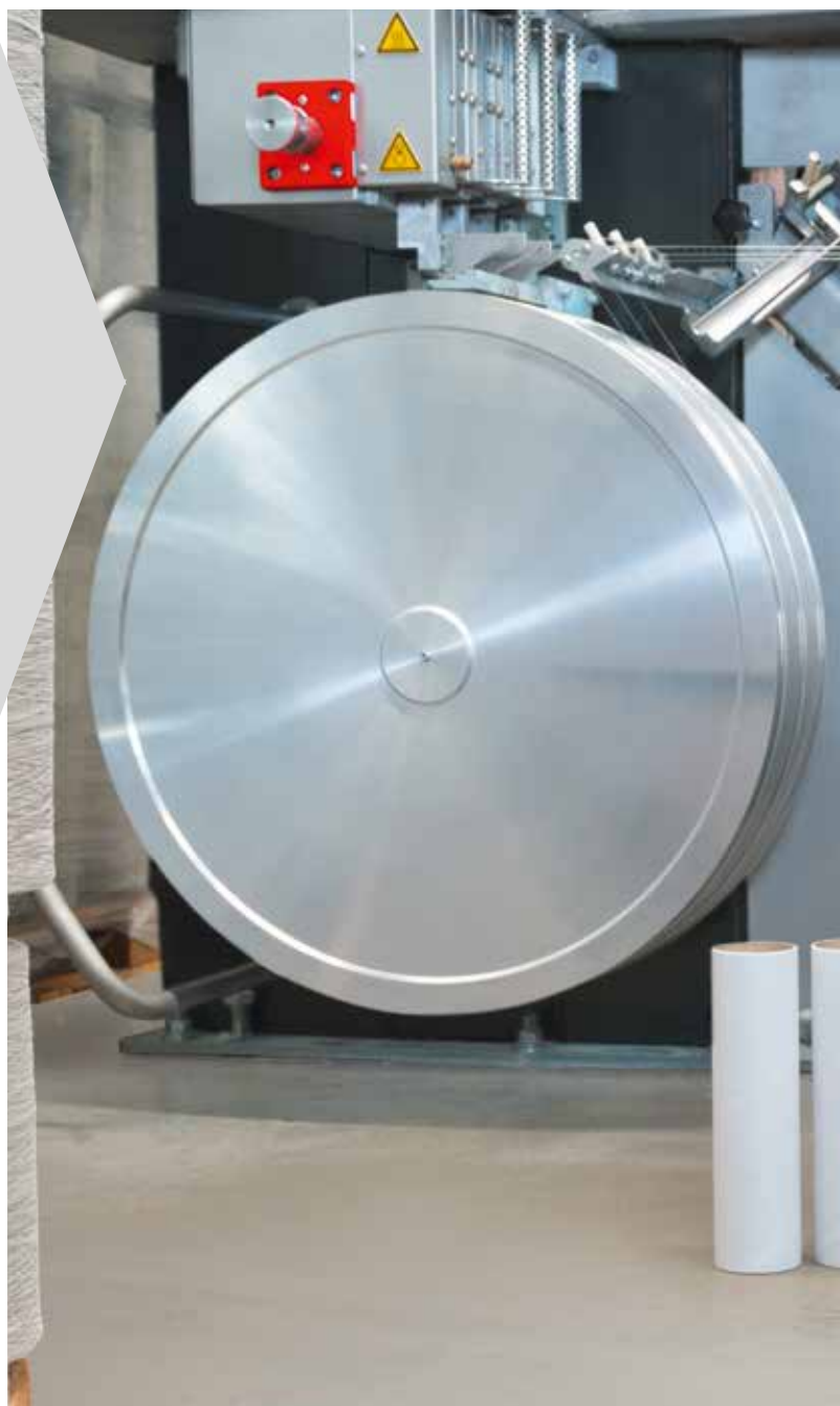
With the new winder Witras III-37, the process speed can be increased up to 3700 m/min.
